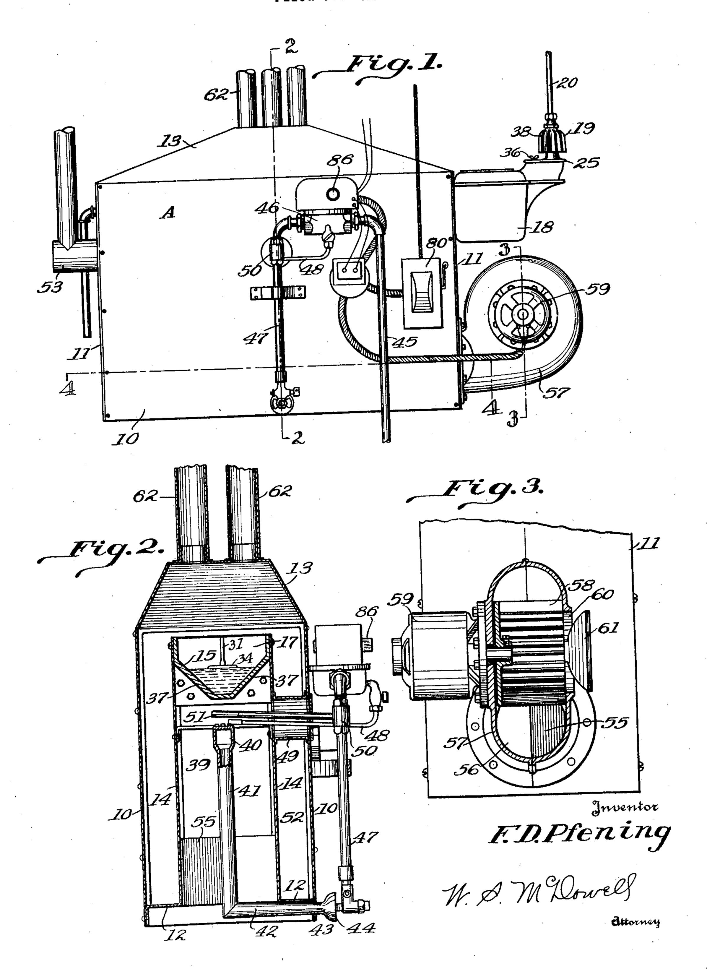
AUTOMATIC HUMIDITY REGULATING MECHANISM FOR HEATING SYSTEMS
